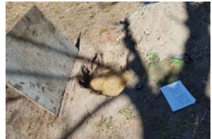
Site 3 hardpan was encountered, and no infiltration took place.
