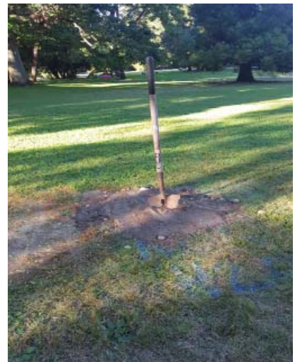
Site 4 soils consisted of sandy loam which made for better infiltration.
